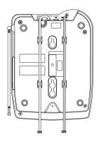
Place the Base Unit on the screws and push down until it's firmly seated.
